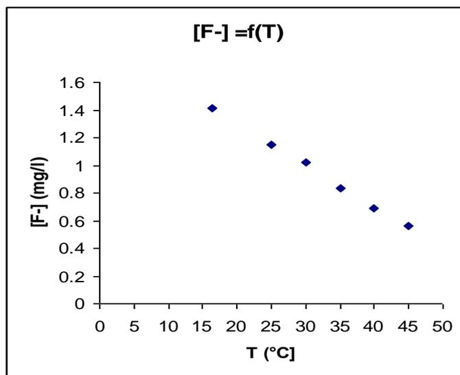
Figure 4. Variation of residual fluoride against temperature.
